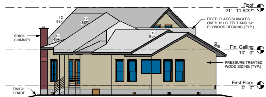
Left (West) Exterior Elevation
